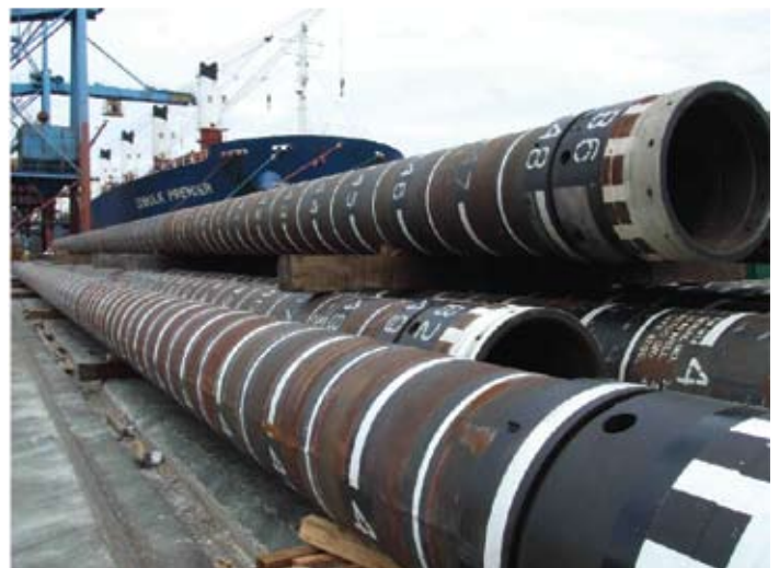
90ft SlimBore wellhead joints installed from a barge offshore Brazil
